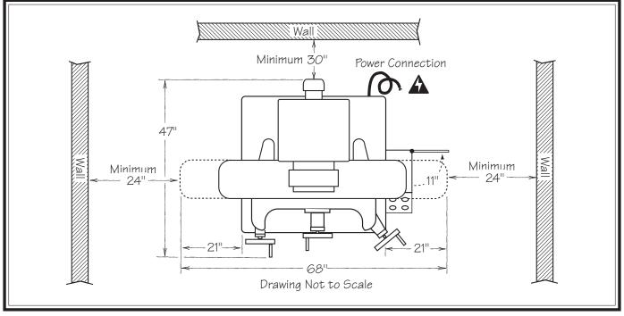
Figure 6. Space required for full range of movement.
